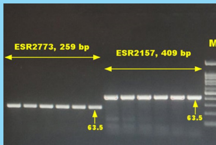
Fig. Agarose gel (2%) electrophoresis of gradient PCR for suitable annealing temperature of primers ESR2773 and ESR2157. M represent 100bp DNA marker. Arrow indicate suitable annealing temperature for respective primers
