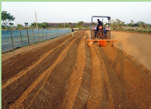
Fig. OFT on Evaluation of Tractor drawn Ridge Former
